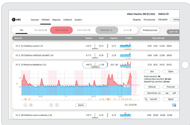
Detail view at the single equipment , you can see the temperature, door opening, defrost time field, door opening statistics...
